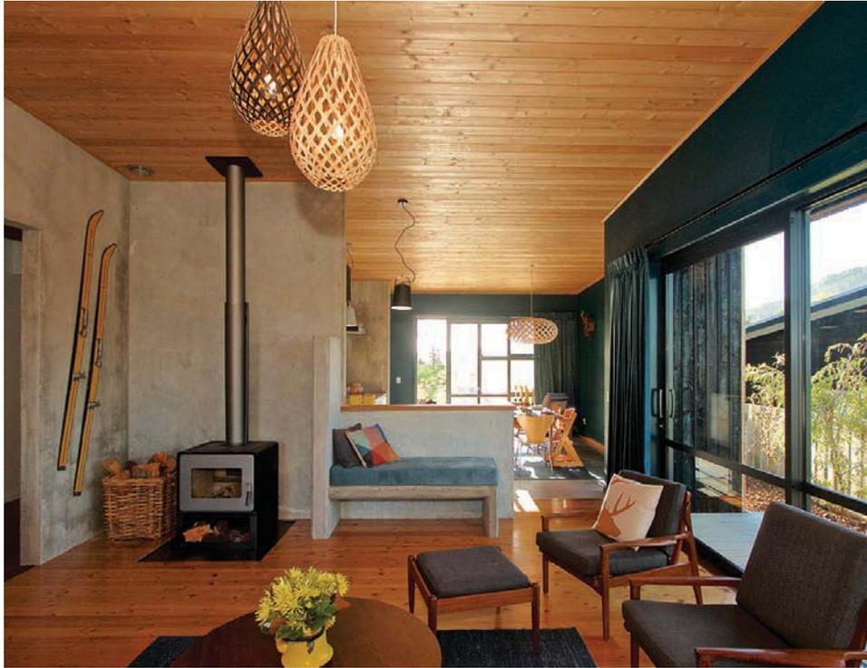
**The 112sqm Kowhai Cabin is airtight making for a snug, healthy home. The sun passively heats the home via concrete slab flooring and concrete tilt panels.**
